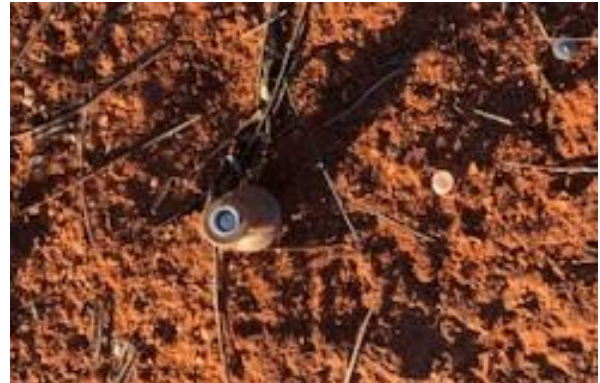
CPE that has been fired - poison capsule broken
